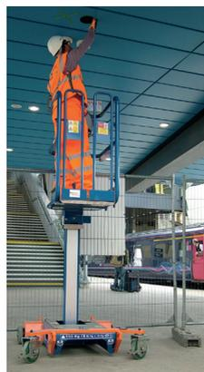
Pecolift Wind Rated is operable on gradients up to 3° and in winds up to 12.5m/s
