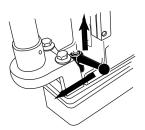
2. With the Clamp Handle Assembly now down, push the Clamp Handle Assembly counter clockwise.
