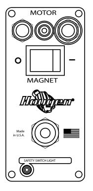
IMPORTANT: Before turning on the machine, it is important that the operator understands the interrelated functions of the SAFETY SWITCH, MAGNET SWITCH, AND MOTOR SWITCHES.
